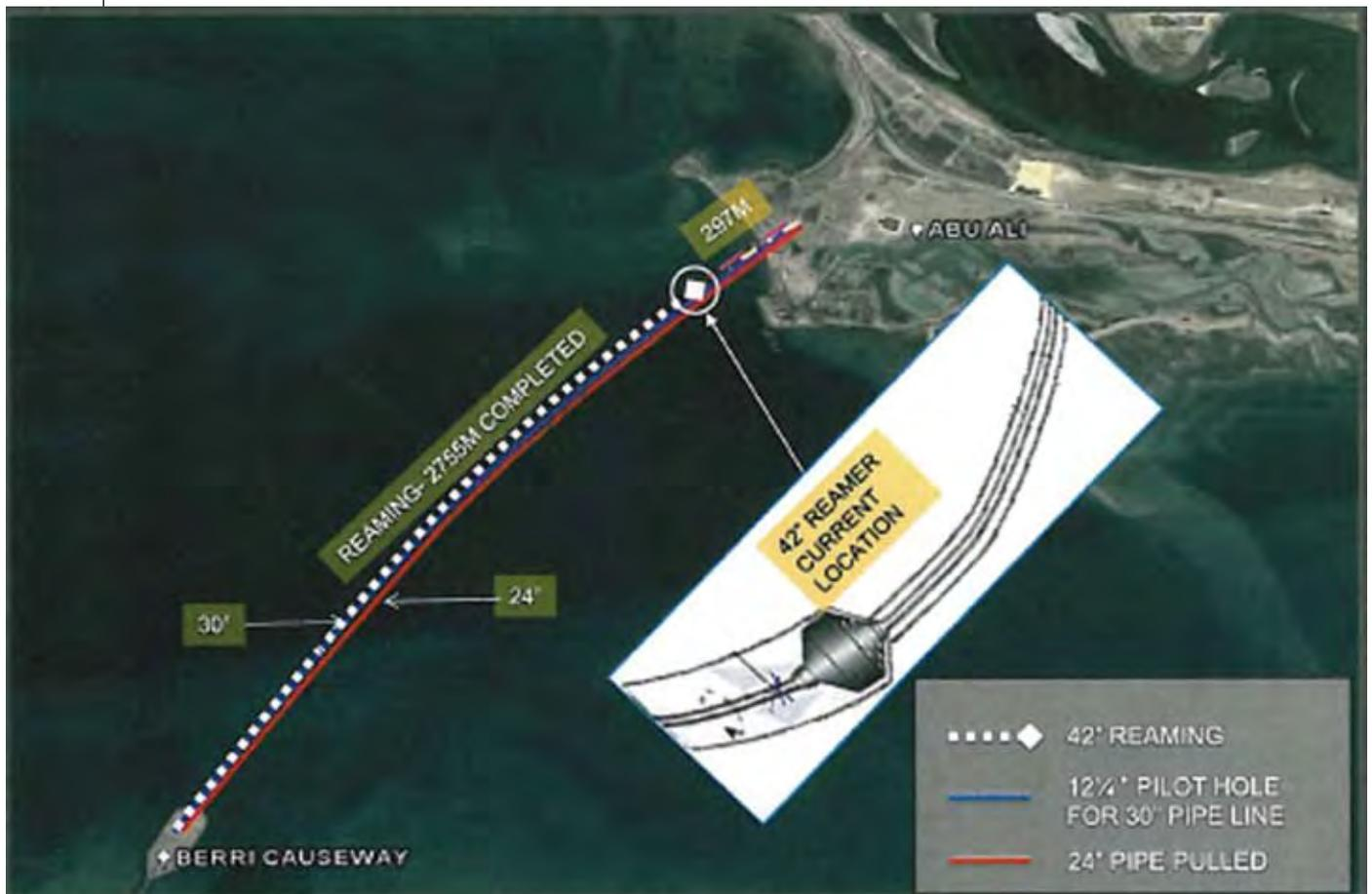
In November 2008 TT-UK were contacted by the Middle East specialist HDD Contractor Digital Connection Co Ltd of Al-Khobar, Kingdom of Saudi Arabia (KSA). They sought technical advice and assistance in the recovery of a 42" hole-opener that had become stuck along with the 3 km drill string beneath the seabed during a pre-ream pass on the second of two under sea pipeline crossings.
