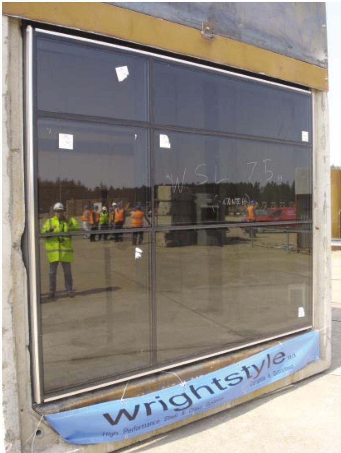
Wrightstyle, based in Devizes, is one of Europe's most innovative steel glazing specialists. Lee Coates is the firm's technical manager and here explains how the company has made a major breakthrough in blast-proof glazing.
