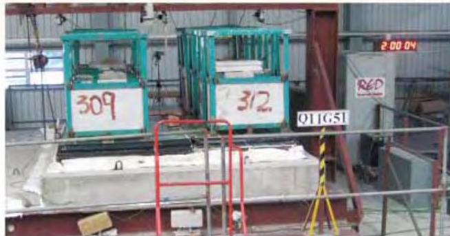
Loadbearing Fire Test at RED 120 mins Insulation, Integrity and Stability according to BS476 Part 20 & 21 : 1987
