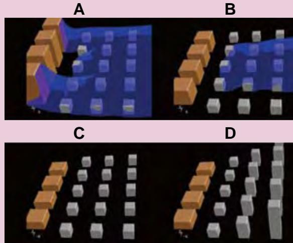
Impact of building configurations on air ventilation (blue feature represents undispersed pollutants) (Source: Fung 2007)
